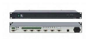
The VP-6A is a high-performance distribution amplifier for computer graphics video signals with resolutions up to and exceeding UXGA and balanced or unbalanced stereo audio signals. It takes one input, provides correct buffering and isolation, and distributes the signal to six computer graphics video outputs on 15-pin HD connectors and one AV twisted pair output on an RJ-45 connector.
