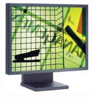
The 20" touch screen LCD NEC 2080UX is an LCD monitor with a touchscreen overlay installed. With single-touch technology, the touchscreen is embedded in the LCD so that when a user touches the screen, it precisely senses the touch location and relay that information to the computer via an attached 6' USB cable.
