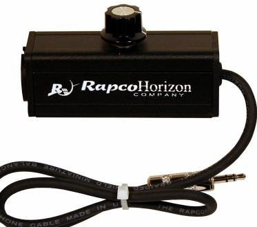
The LTIBLOX is a consumer to pro interfaces. It converts input from consumer grade equipment (laptop computers, MP3 players, CD players) to a mic level balanced output. It also gives operator volume control of the outgoing stereo signal. 3.5mm male input and XLR male output.
